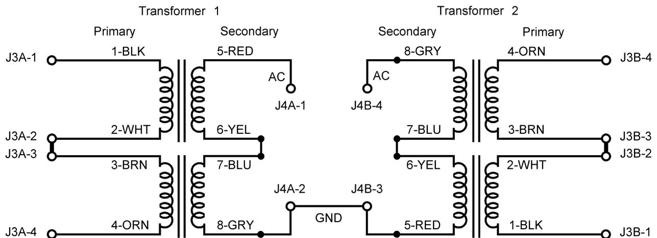
**Figure 3. 120V Transformer Connections, Primaries in Series**
