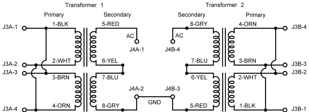
**Figure 2. 120V Transformer Connections, Primaries in Parallel**
